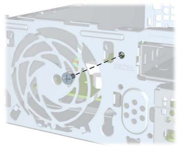
Figure 7-8 Retrieving the Front Bezel Security Screw
